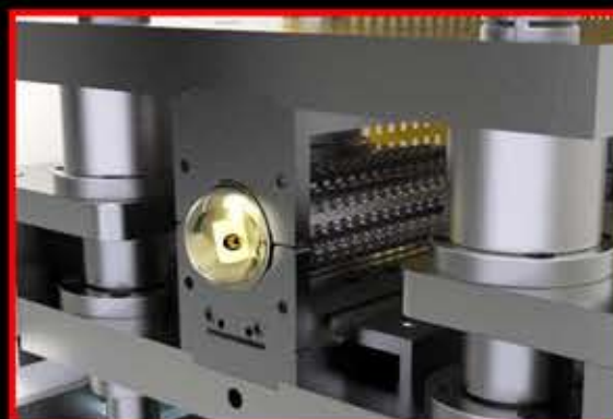
Top and bottom tube clamp plates open and close simultaneously for every transitional movement
