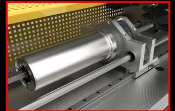
Collet chuck with hydraulic clamping for positive grip
