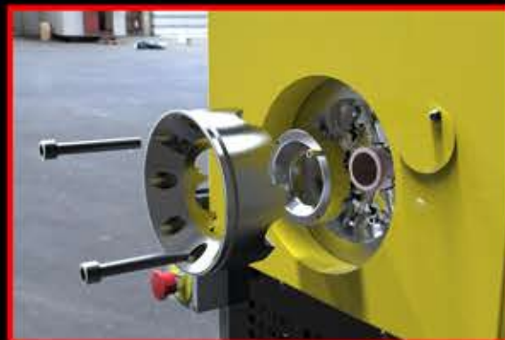
Head tooling can be changed by removing just two bolts, with a full tool change (including mandrel) in under 10 minutes
