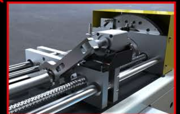
An air ram provides strong clamping of the chuck around the tube while also eliminating the need for hydraulics
