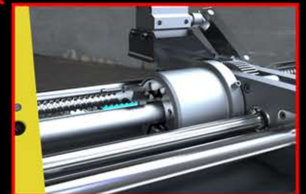
A new collet design allows the collet inserts to be swapped without removing the shroud decreasing tool change time
